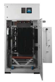
The Automatic Transfer Switch is installed on a draw-out mechanism, with electrical and mechanical interlocks for secure removal after load bypass. The ATS control/logic panel is mounted on the enclosure door and connected by a wire harness and multi-pin disconnect plugs. The transfer switch and/or the control panel may be tested, isolated and removed for maintenance without load interruption.
